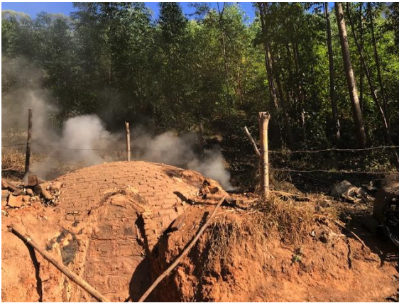
Old fashioned kiln - Hillside Kiln ("forno de encosta")
