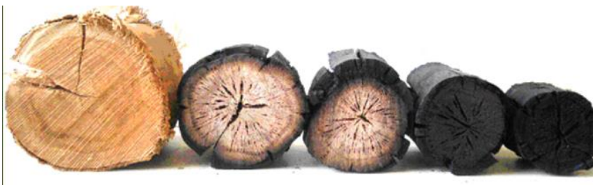
Figure 3 - Wood carbonization process
