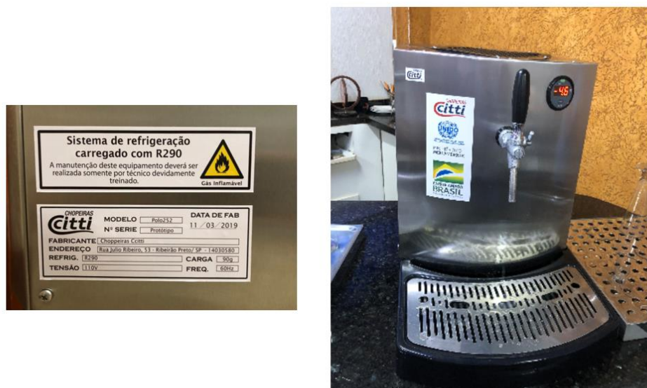
Figure 1 – Draft beer cooler equipment developed under the RAC Project, March 2019.
